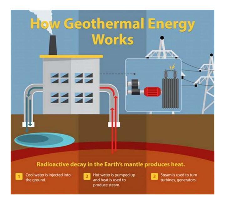
Geothermal energy utilizes heat from beneath the Earth's surface to generate electricity or provide heating and cooling. This renewable energy source offers a reliable and constant power supply, with minimal environmental impact.
