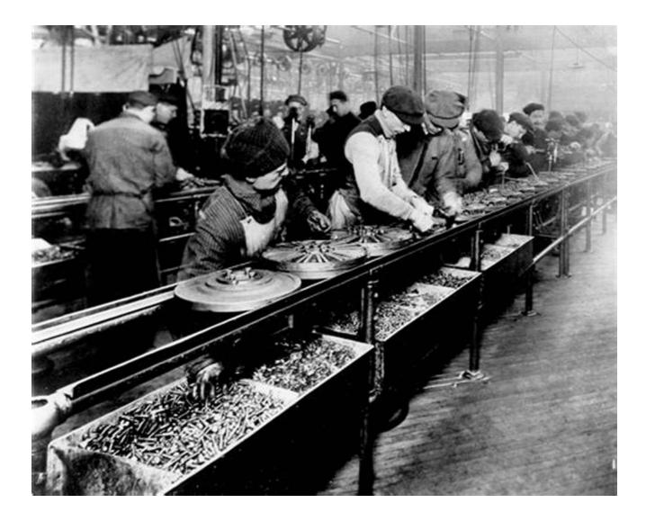
Henry Ford's of the assembly line in the early 20th century may be more commonly associated with mass production, but its roots trace back to the Industrial Revolution. The implementation of division of labor and mechanized processes in factories significantly increased productivity and reduced production costs. This breakthrough heralded the era of mass production, enabling the creation of goods on an unprecedented scale and making them more affordable for the general population.
