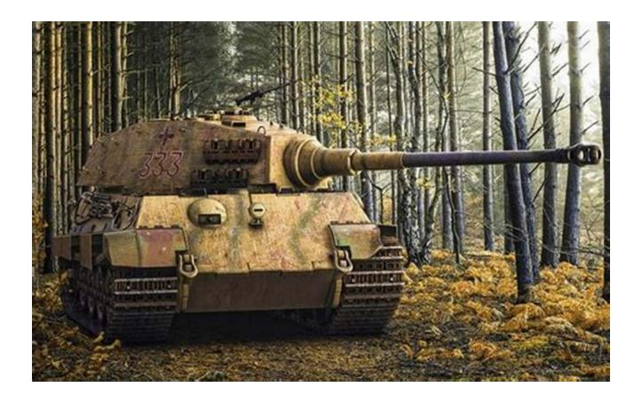
The Tiger II, also known as the King Tiger, was Germany's response to the increasing armor thickness of Allied tanks. It featured incredibly thick frontal armor, making it almost impervious to most Allied anti-tank weapons. Its high velocity 88mm gun could easily destroy enemy tanks from great distances.
