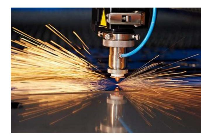
With their precision and high power, lasers have revolutionized the manufacturing industry. Laser cutting involves the use of a highly focused laser beam to cut through various materials such as metal, plastic, and fabric. Laser welding, on the other hand, utilizes the heat generated by the laser beam to create strong and precise welds. These applications have significantly improved the speed, accuracy, and efficiency of manufacturing processes.
