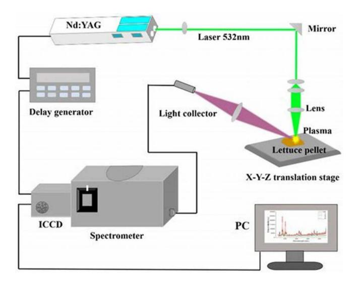
Laser-Induced Breakdown Spectroscopy (LIBS) is a powerful analytical technique used to identify and analyze the elemental composition of substances. It involves focusing a high-energy laser beam on a small area of the material, resulting in its breakdown or vaporization. The emitted light is then analyzed using spectroscopy to determine its elemental composition. LIBS finds applications in metallurgy, forensics, environmental analysis, and even planetary exploration.
