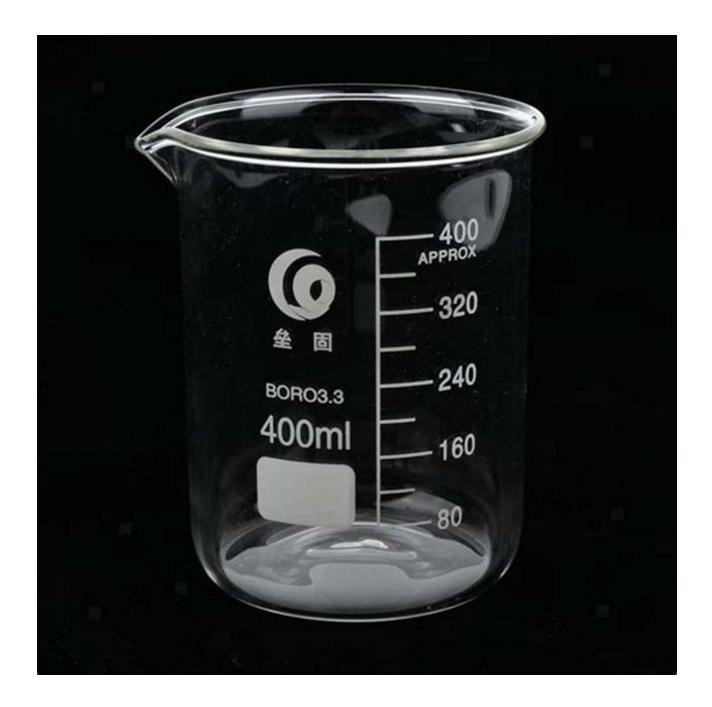
The beaker is a staple in every chemist's lab. It comes in various sizes and is used for mixing, heating, and measuring large volumes of liquids. Whether they are concocting colorful solutions or carrying out titration experiments, chemists rely on the mighty beaker to stir up astonishing reactions!
